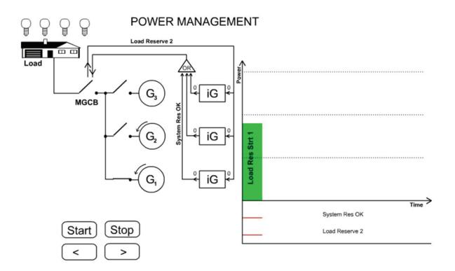
**Phase 2:** According to load demand, necessairy number of generators keep working (in this case it is 2 generator sets)
